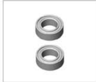
PV0176 BALL BEARING, d4xD7xW2.5
